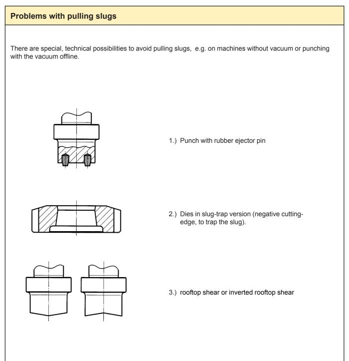
The problem can eventually be cleared when the punch goes past the grind life approx. 1 - 2 mm deeper into the die.
