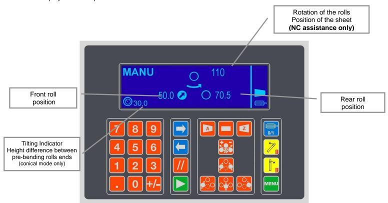
In manual mode, the tilting of rolls is enabled for conical bending. The tilting angle is set by the cone potentiometer and the current value of the tilting is displayed on the left bottom corner of the screen.
