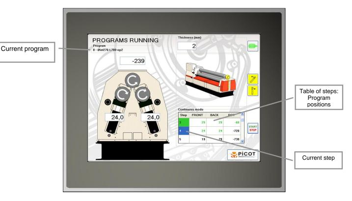
In the case of serial part production, the first sheet is made manually: the NC records automatically each stages of the manual forming process into a program.
