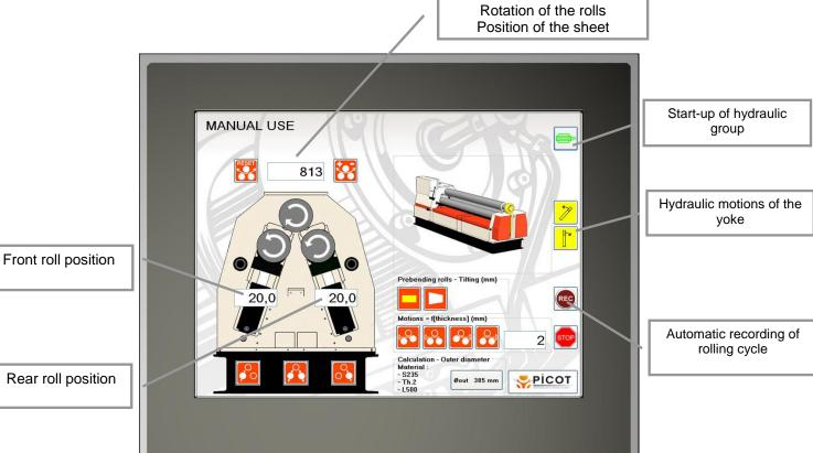
Rolls motions driven by touches on the screen are automatic motions which allow the operator to go directly to the target position. 556
