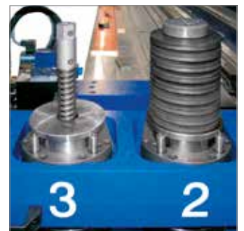
Maximum tool size of 88.9 mm diameter
