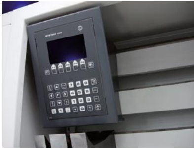
Second monitor in the tool magazine
