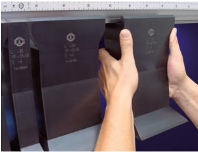
The UpDownBend clamps the upper beam and folding beam tools automatically
