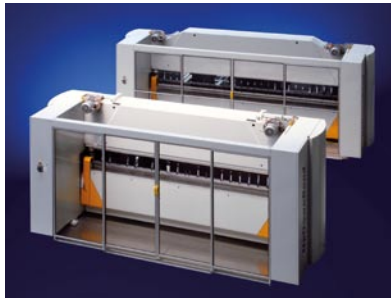
Glass sliding doors secure the folding area
