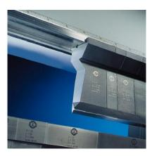
Automatic upper beam tool clamping system
