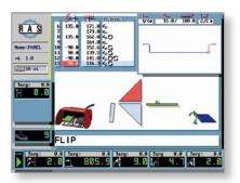
After the program is started, the graphic shows the operator which foot pedal he needs to press. Operator instructions such as "Flip" or "Paint up" allow even inexperienced operators to produce perfect parts.
