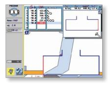
If a collision has been analyzed, the control displays this situation graphically. Technology tables consider material springback. The calculated blank dimensions are automatically corrected by the bend allowance, used for the radii.
