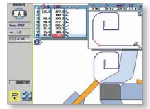
The CADalyzer calculates several folding sequences and for most parts automatically creates a program. The simulation shows the program, the finished part and the actual bend sequence.
