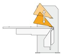
Programmable upper beam position during clamping and unloading
