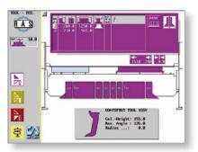
The setup instruction displays which tool segments are required for the length of the part. This information is available for the upper beam, the folding beam and the lower beam. For easy setup, the Touch&More graphically displays the tool shape.
