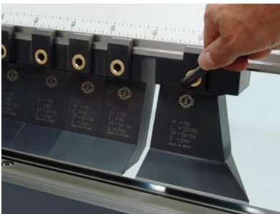
With the quick clamp system, tools can be changed in seconds
