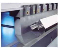
The boundless front and side free space can accommodate return flanges up to 56 mm (2 165")
