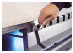
With the quick clamp system, tools can be changed in seconds. The tool seat is integrated directly into the upper beam.
