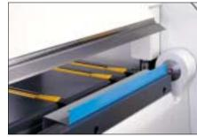
Sheet support panels moved backwards to accommodate reverse flanges
