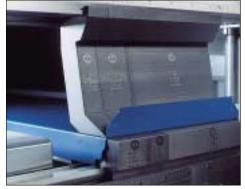
Segmented lower beam tooling for reverse flanges of up to 40 mm (1.575").
