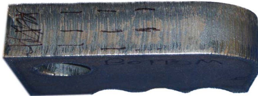
Figure 2: 16 mm Fiber Laser Cut Mild Steel
